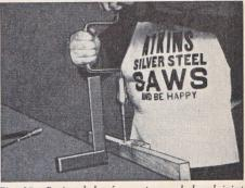
Fig. 27-Boring holes for a staggered dowel joint
