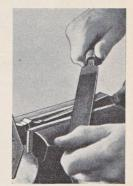
Fig. 47—Draw-filing brass candlestick before polishing
