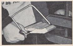
Fig. 35—Using the ATKINS Silver Steel Coping Saw No. 100 to cut moulding for a coped joint
