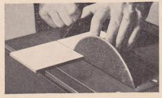
Fig. 58—Cutting asbestos composition tile with Bakelite Bonded Wheel on circular saw table
