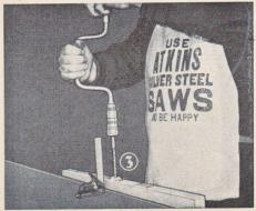
Fig. 24—Boring holes to make a plain mortise
