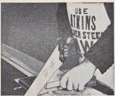
Fig. 18—Cutting a mitre joint with ATKINS Silver Steel Panel Saw No. 53
