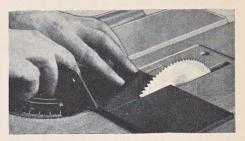
Fig. 53-Circular Saw Cutting Bakelite panel
