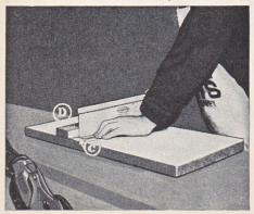
Fig. 15—Making cut in stopped dado joint, with ATKINS Silver Steel Back Saw
